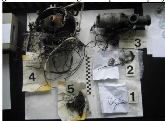
Figure 7. Excluded samples from the engine compartment of buses for laboratory analysis
