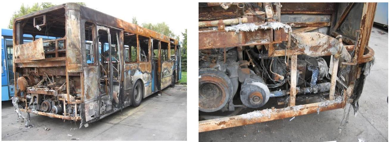
Figure 6. Buses and engine compartment after fire
