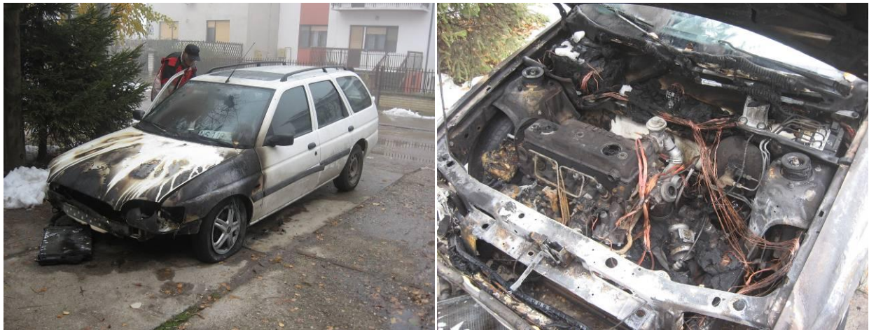
Figure 5. The vehicle and the engine compartment after fire
